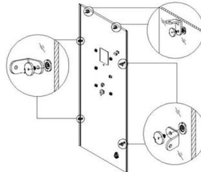
8. Place bottom edge of glass A into the slot on the base as shown. A small amount of soap or lubricant on the gaskets will help with installation.
