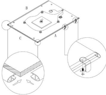
15. Insert the rubber seals into the movable glass door and attach. *Note: Read the Door Installation Help.*
