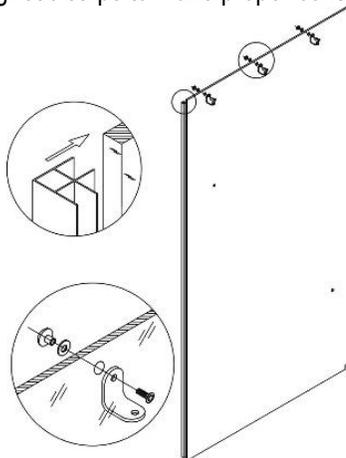
6. Insert the half-moon shaped rubber seals on both sides (outside facing edge), and top edge of glass A. Note: top gasket may be already installed on the control panel.
