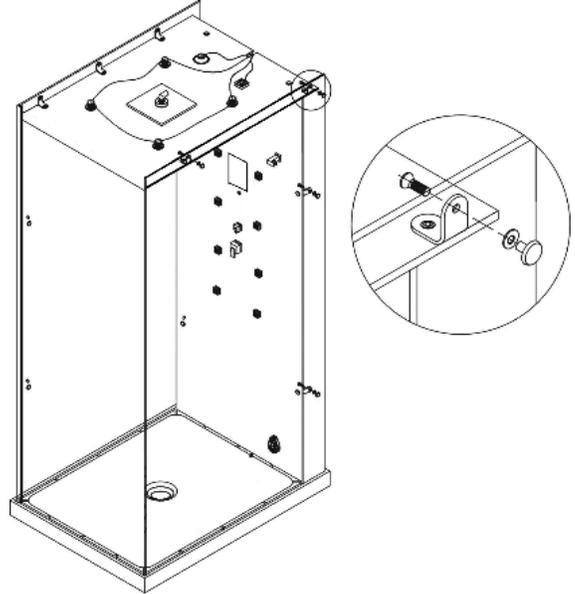
13. Place glass C into the slot onto the base and insert into the corner seal of glass B. Note: Glass C is the clear panel, and glass B is a black/white large solid panel. Line up the installation holes and connect glass B and glass C. Note: Use Windex for lubricant.
