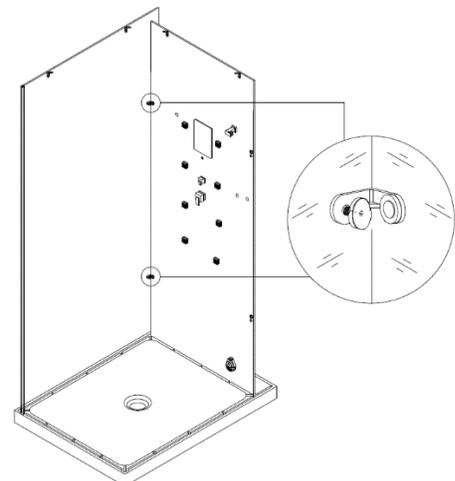
9. Electrical Connections: The wires for the fan, speaker, and light are labeled. Make the corresponding connections from the accessory to the wire coming from the control box. \*Note: Be cautious when making this connection. The pins of the connector can easily bend if connected improperly!
