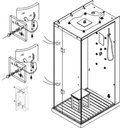
17. On the hinge side, install the half moon gaskets and the handle side, install the magnetic gaskets
