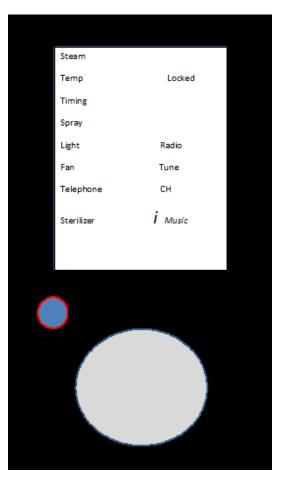
The Mhz will be displayed. To Manually find a station Make sure the Mhz is flashing by making sure the tune is highlighted and pressing Shuttle Knob. The Mhz will start to flash then you can then rotate the Shuttle Knob to the particular station. Once you have found your particular station press the Shuttle Knob to set it.
