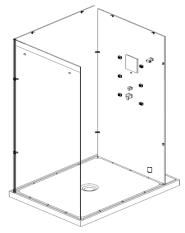
16. Make sure the half-moon shaped seals are on the sides of the top D. If needed, assemble the half-moon shaped seals on the sides A, and C of glass D (top). See illustration. Attached angle brackets to glass panel D. Note: The fan and speaker side of the glass will hang over the main control panel.
