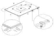
17. Place glass D (top) on the top of the unit, align connecting holes with glass D to glass panels A, B and C. Use connector bolts to connect. Refer to illustration.
