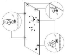
15. Slide panel A into the corner gasket on panel B. Secure the two panels with the 90-degree brackets. Small amount of lubricant on the gaskets will help with installation.
