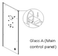
Install angel brackets over the installation holes of glass A, connect with connector bolts (make the connection snug, but loose enough to make adjustments.)
