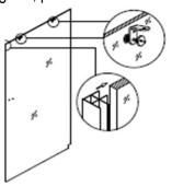
11. Note: Use Windex for lubricant. Slide glass C into the open side of the corner gasket on glass B.
