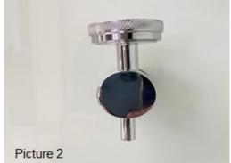
Valve is closed for Steam Generator Operation
